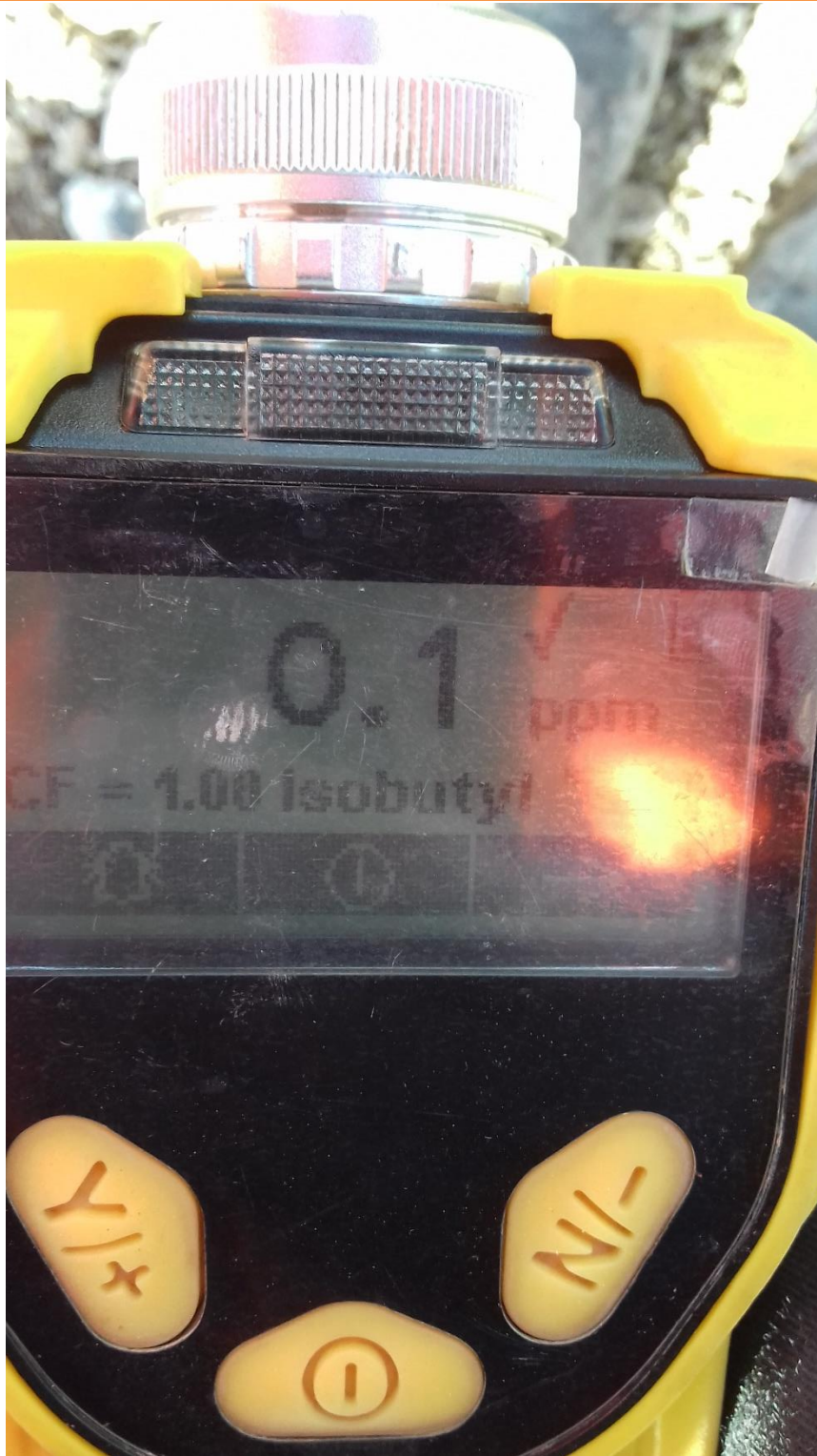
PLATE 21 – SCREENING OF MATERIALS USING PID (MATERIALS <0.5PPM COULD REMAIN IN-SITU)
