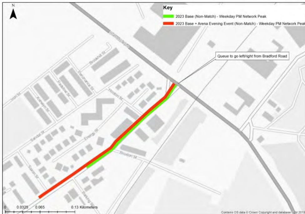
Figure 3: Queues Along Bradford at Hulme Hall Lane/Bradford Road Junction
