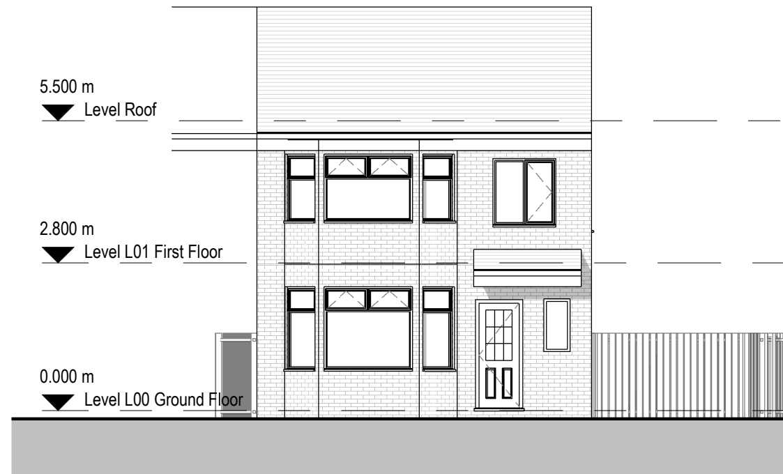
1 Existing West Elevation 1 : 100
