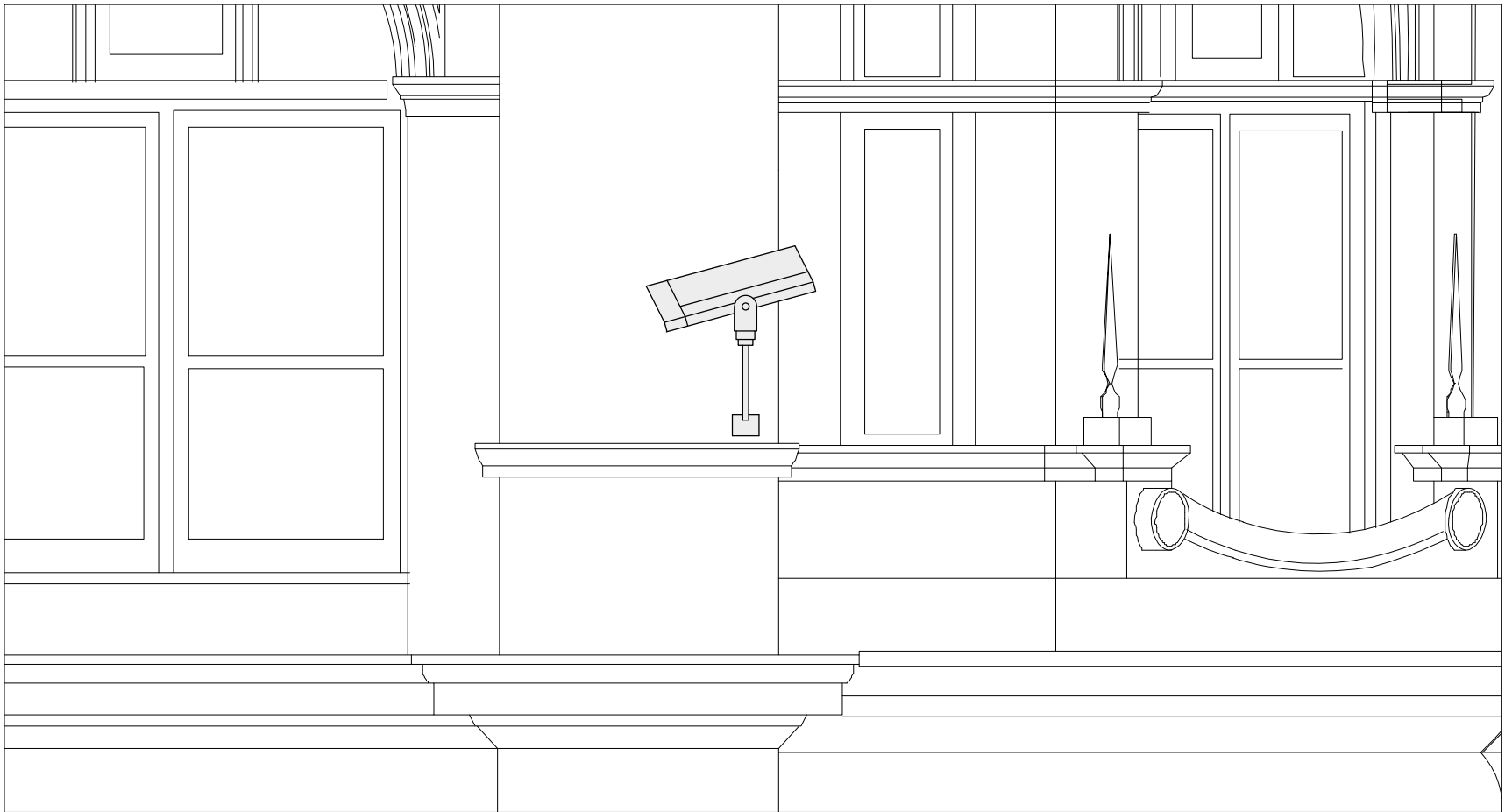
Existing camera 27 to be replaced (front view) Esc. 1:25
