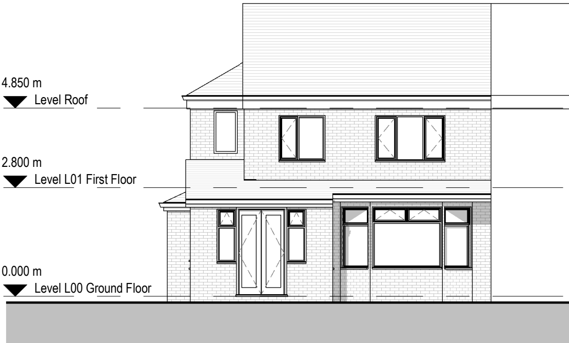
1 Proposed North Elevation 1 : 100
