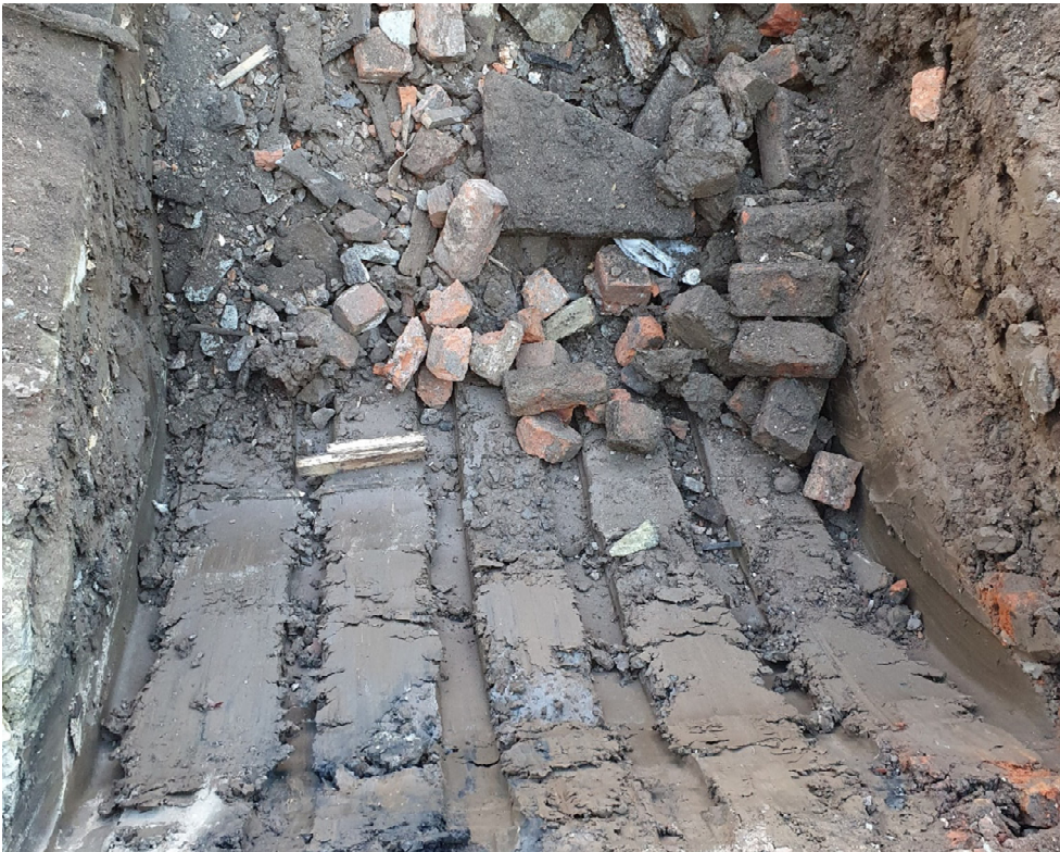
Photograph 4 - Natural soils exposed beneath basement in TP102
