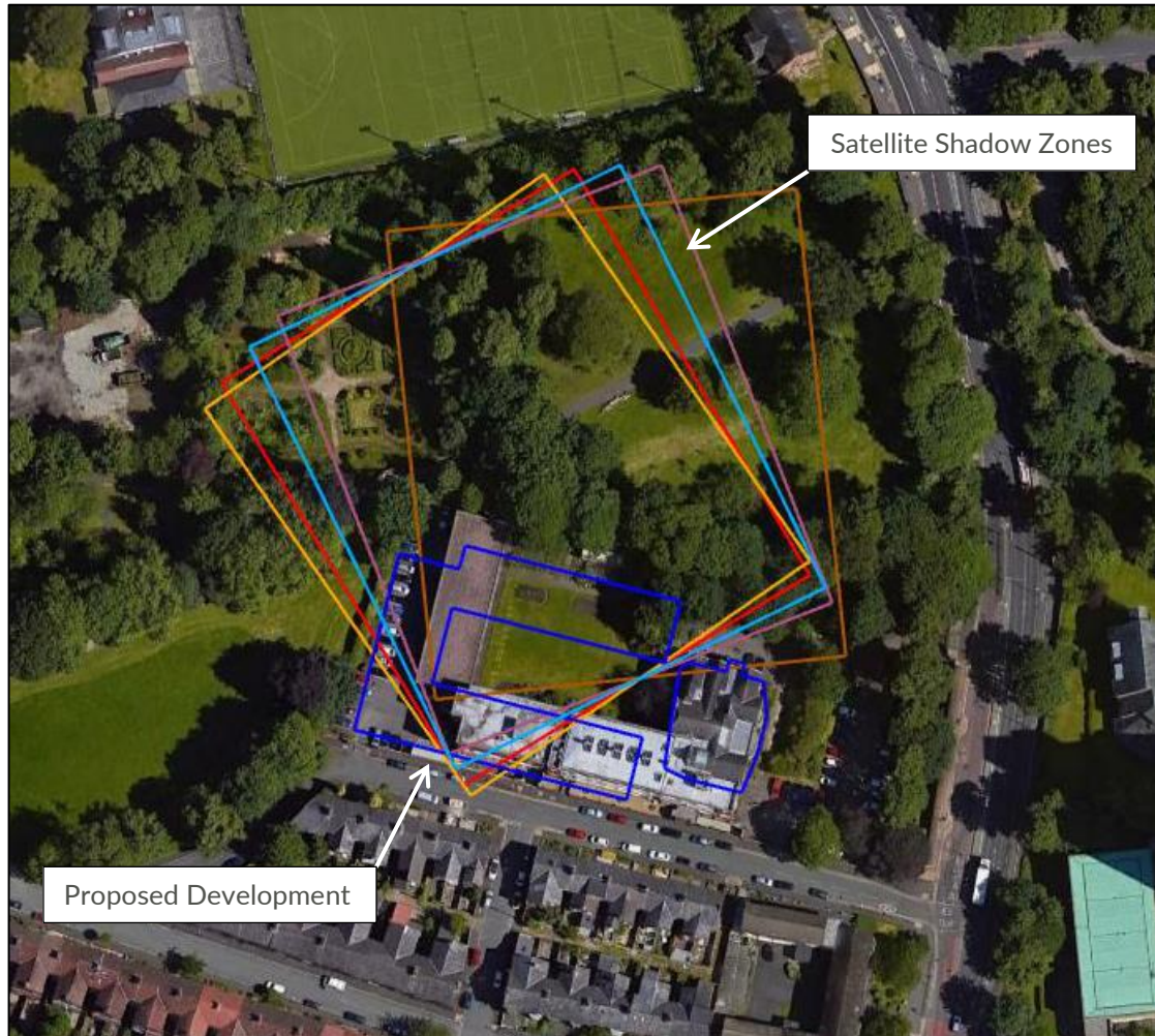
Figure 10 Terrestrial television interference zones (aerial image)
