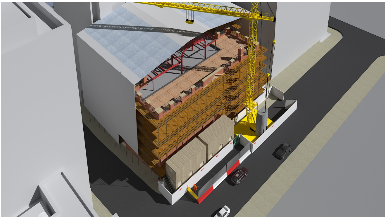
Image showing the site set up with tower crane, full height scaffold (will be sheeted) and the pit stop area in front of the hoarding for unloading materials
