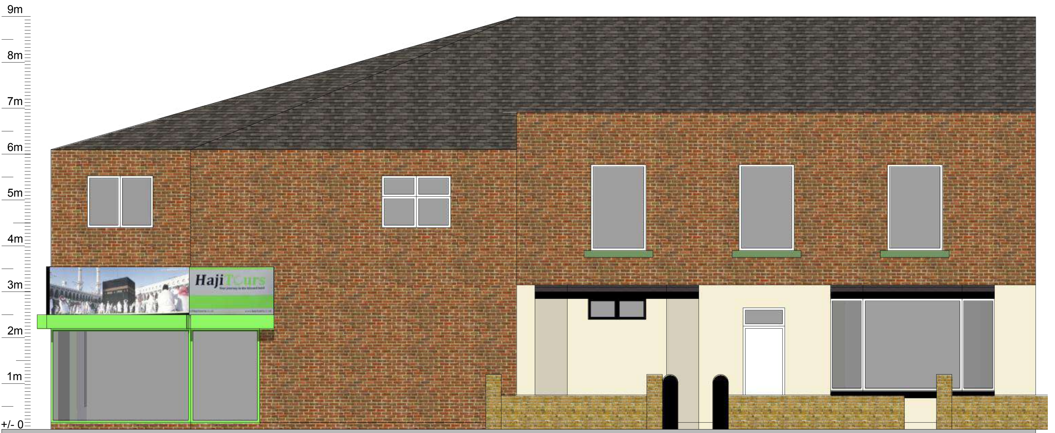
PROPOSED: SIDE ELEVATION SCALE 1:50
