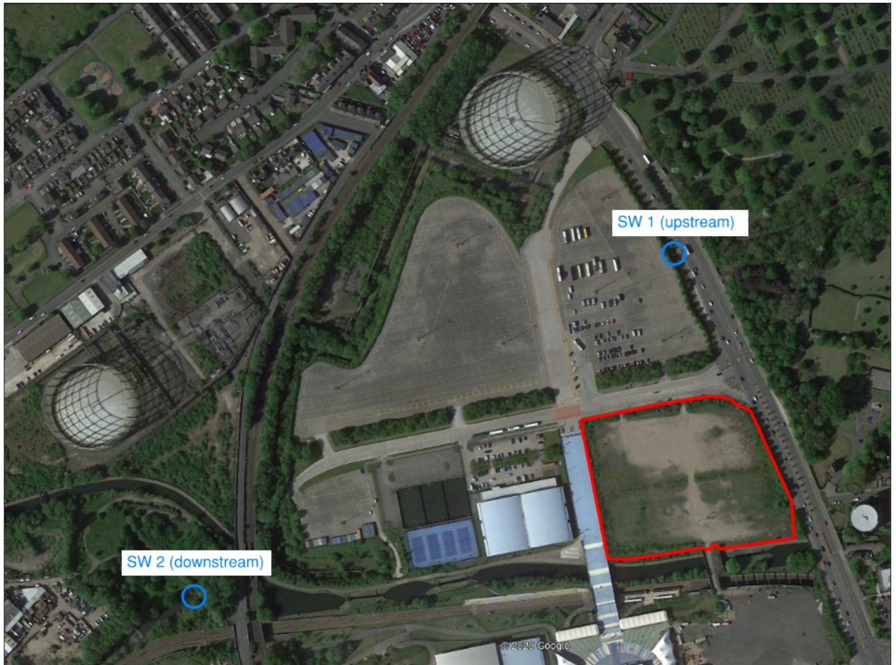
Figure 2 Extract from Google Earth showing surface water monitoring points (entrance and exit to the culvert) up and down stream of the site.
