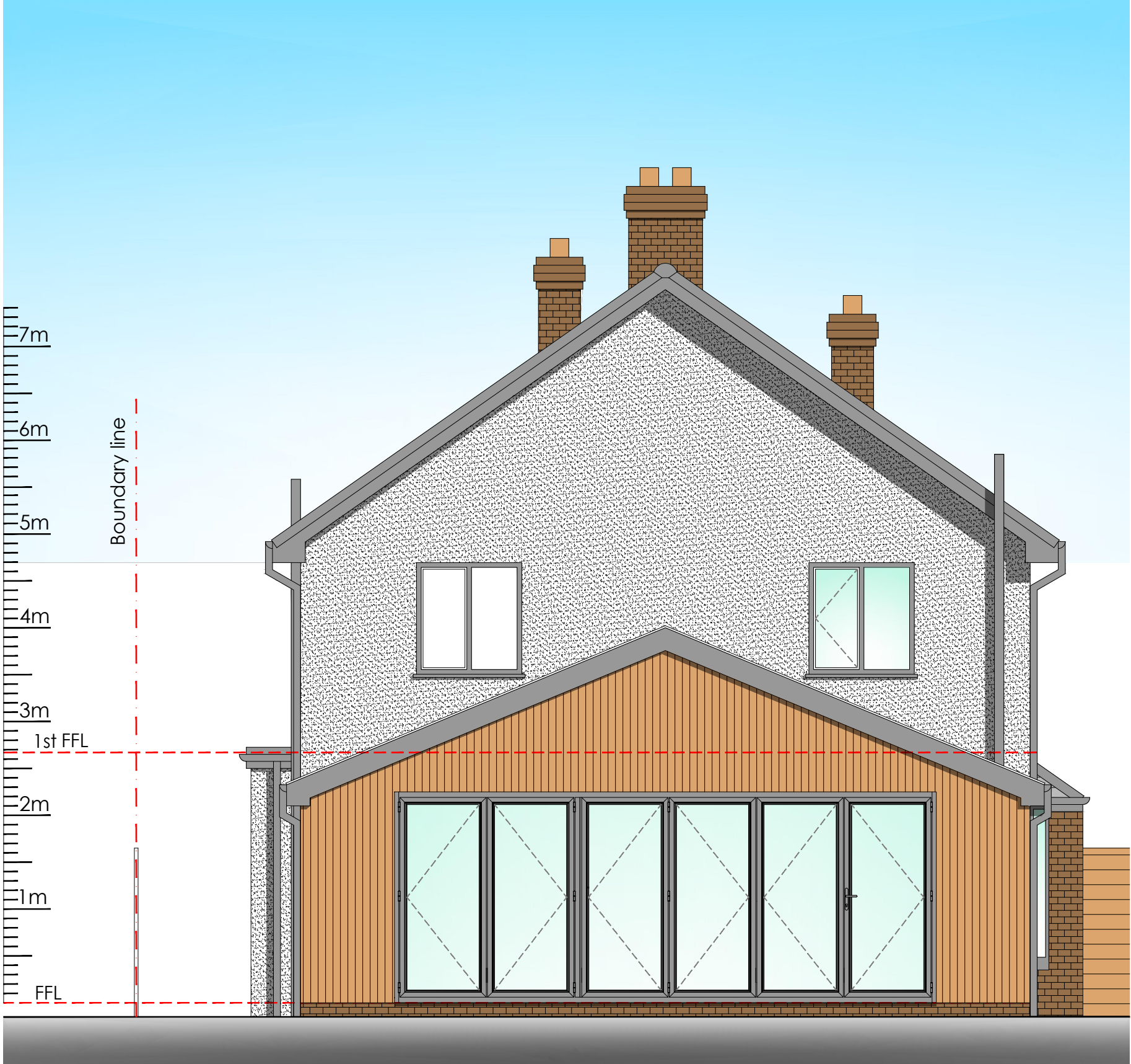
side elevation - as proposed scale 1:50 at A1
