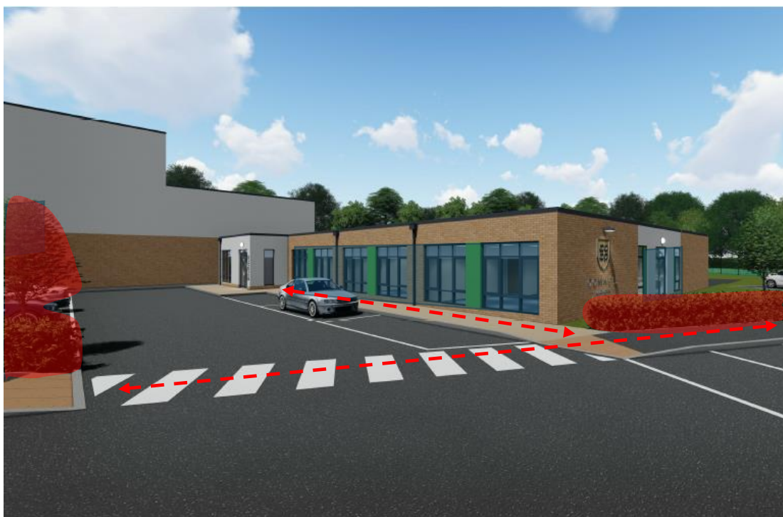
Examples of CPTED highlighted; Signage and wayfinding, landscaping and good Natural Surveillance from ground-floor windows
