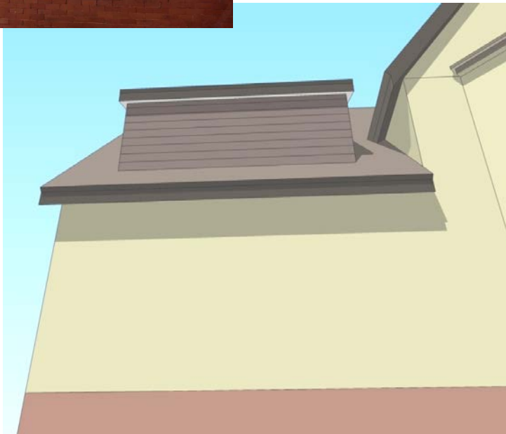
Proposed shed dormer to side elevation roof
