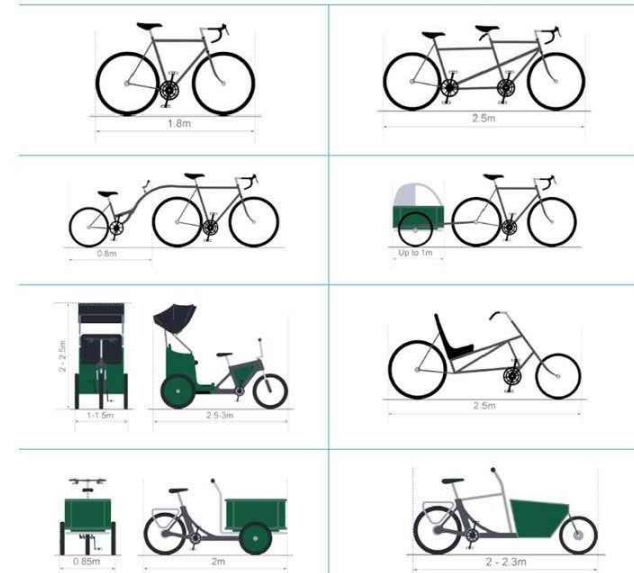
Figure 5.2: Typical dimensions of cycles
