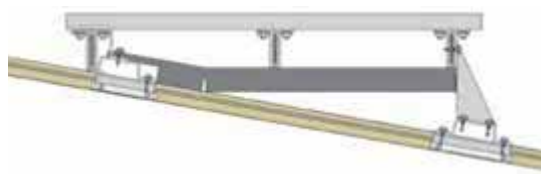
Example detail (note: slate layer not shown) fixed to sarking board.
