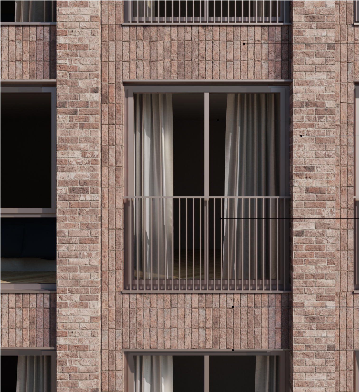
PROPOSED BAY DETAILING 1 - 100MM RECESS ON PIGEON AND LASYTALL ST ELEVS
