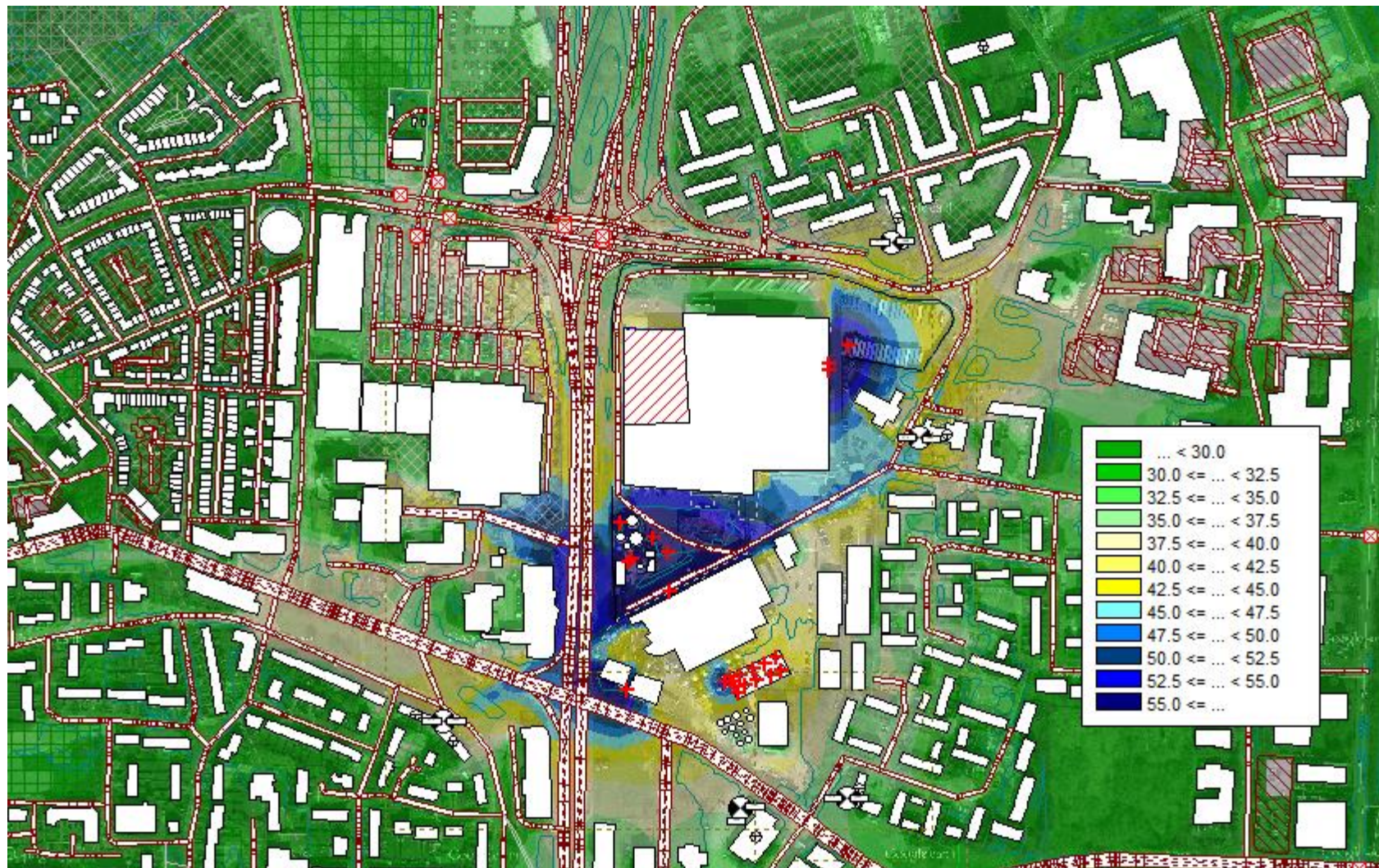
Figure 2 – noise contour map without proposed Maze Silos
