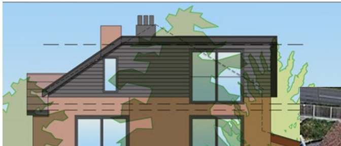
Rear and side elevations Mansard roof
