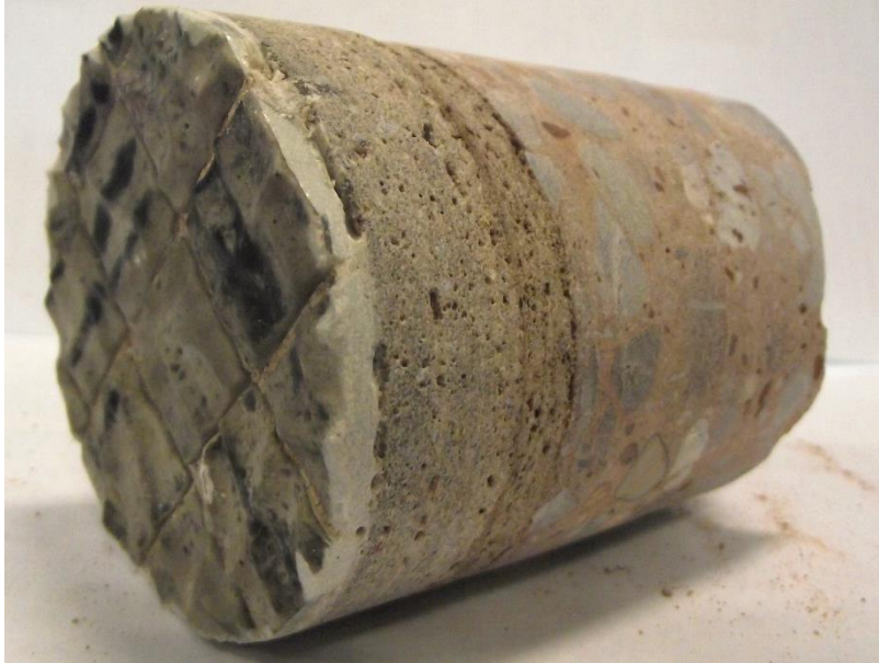
Figure 2.2: Additional core photograph showing the form of the cladding
