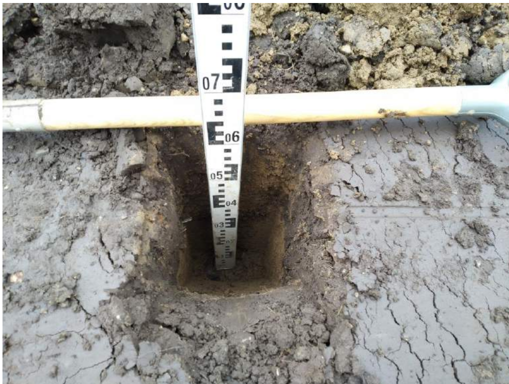
Photograph 11 150mm to topsoil and 450mm of subsoil emplaced in VP02.
