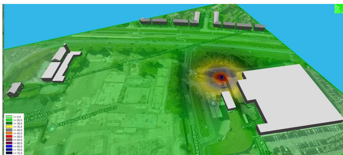
Figure 3 – ISO view of noise emissions from the site (CadnaA); all EV charging services operational.
