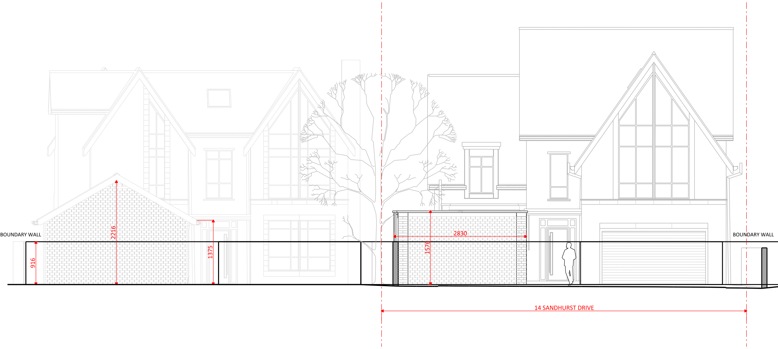
PROPOSED FRONT ELEVATION [BEHIND BOUNDARY WALL] (1:100)
