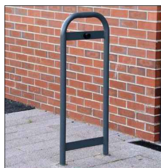
Anti-Trap Bollard/Cane Guard Door Barrier BX14/DB by Broxap. Galvanised and polyester powder coated finish; colour black. Paving core-drilled and barrier root fixed through into concrete foundations.
