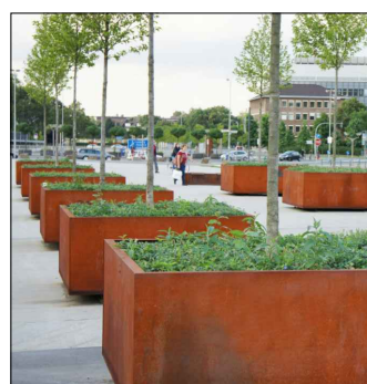
Tree planters to Birchall Way frontage to be Cor/Ten 'ShrubTub' 1200x1200x1000mm by Streetlife NL, or equal and approved.
