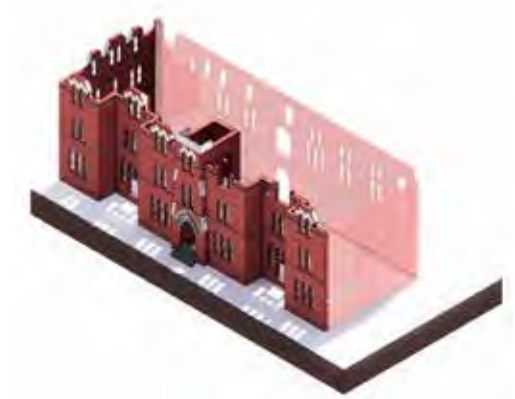
(2) Demolition of façades of lower significance to facilitate safe access for machinery to remove rubble and for access for a piling rig, whilst creating a bigger development footprint
