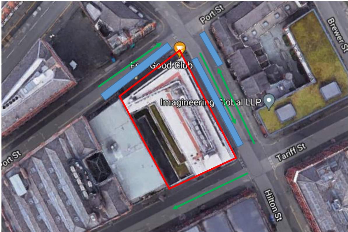
Figure 1 – Routing of construction traffic. Blue identifies on street pay and display parking.
