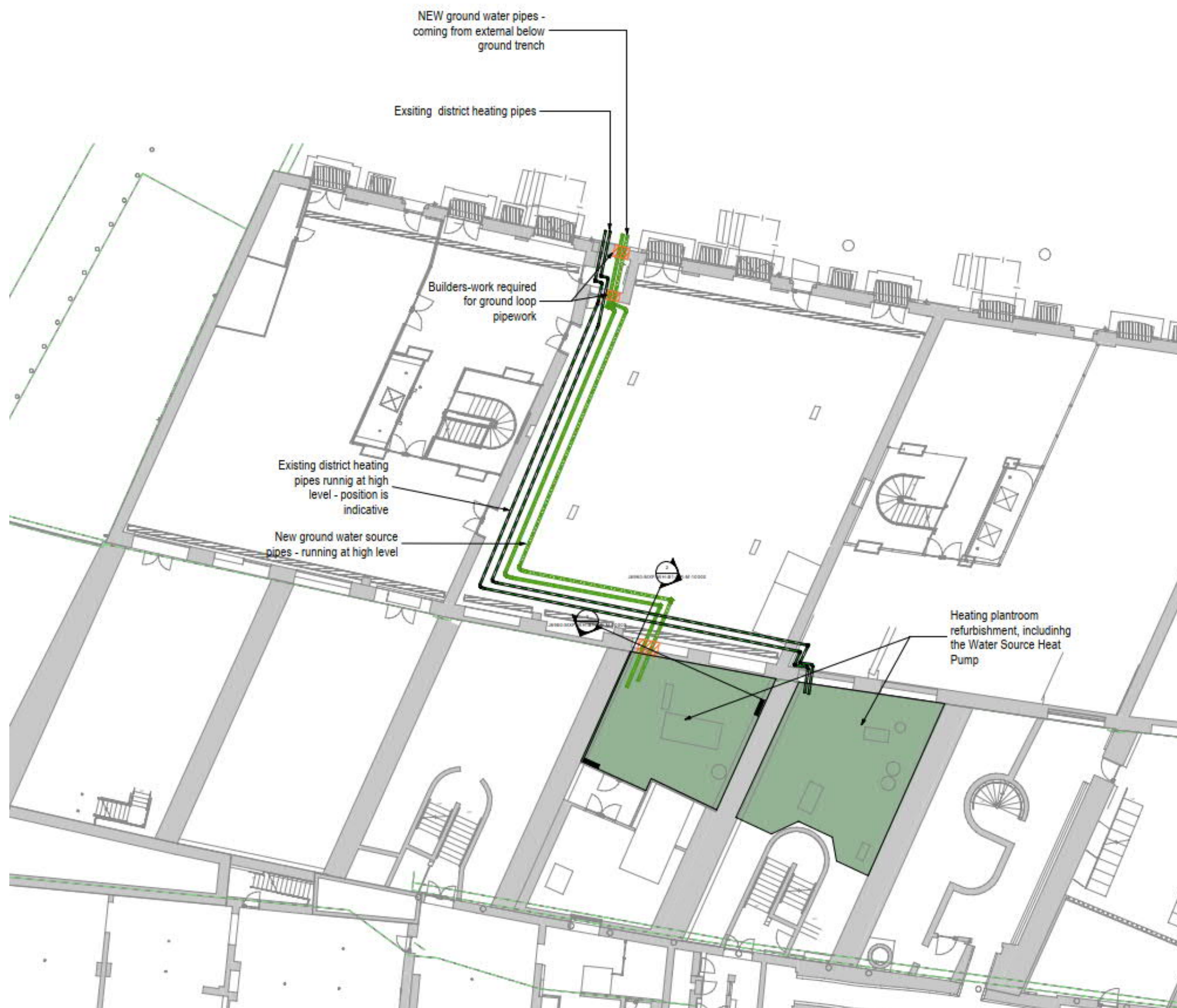
Figure 8-2 - 1830 Warehouse - new GSHP & pipework layout – drawing snapshot - refer to the related drawing for the readable version
