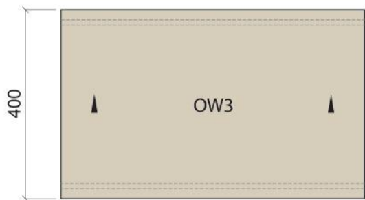
OW3 Once Weathered Coping, 400x75/50mm Section
