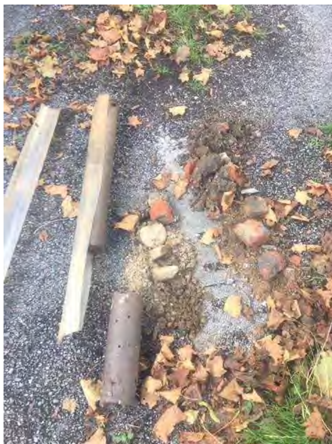
Photograph 8: Arisings from WS3 (1-4mbgl)
