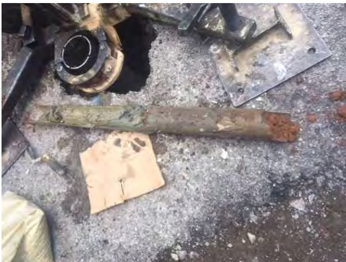
Photograph 6: Arisings from WS1 (4-5mbgl)
