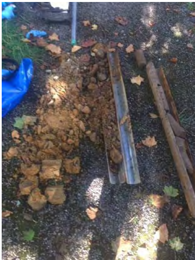
Photograph 7: Arisings from WS2 (1-4mbgl)
