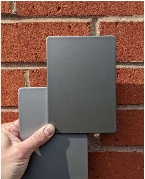
SITE PHOTOGRAPH Proposed ALBOND 9000 (A2) materials against the existing brick
