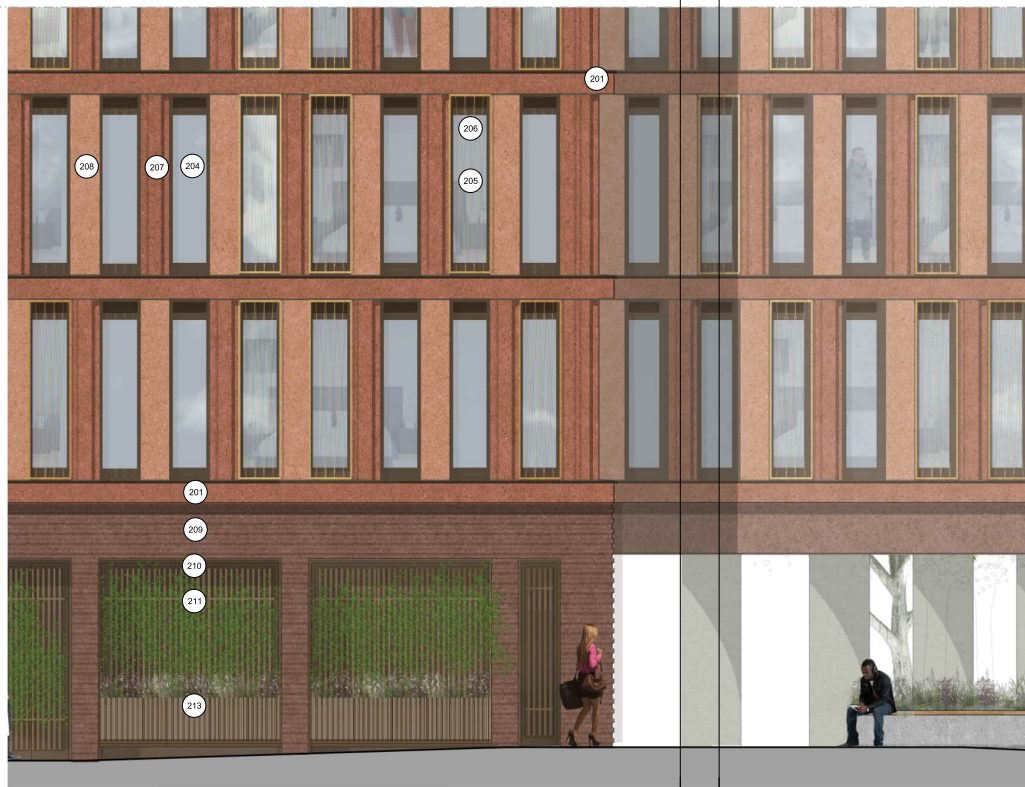
03 South Elevation Reconstituted stone facade - Staggered bays
