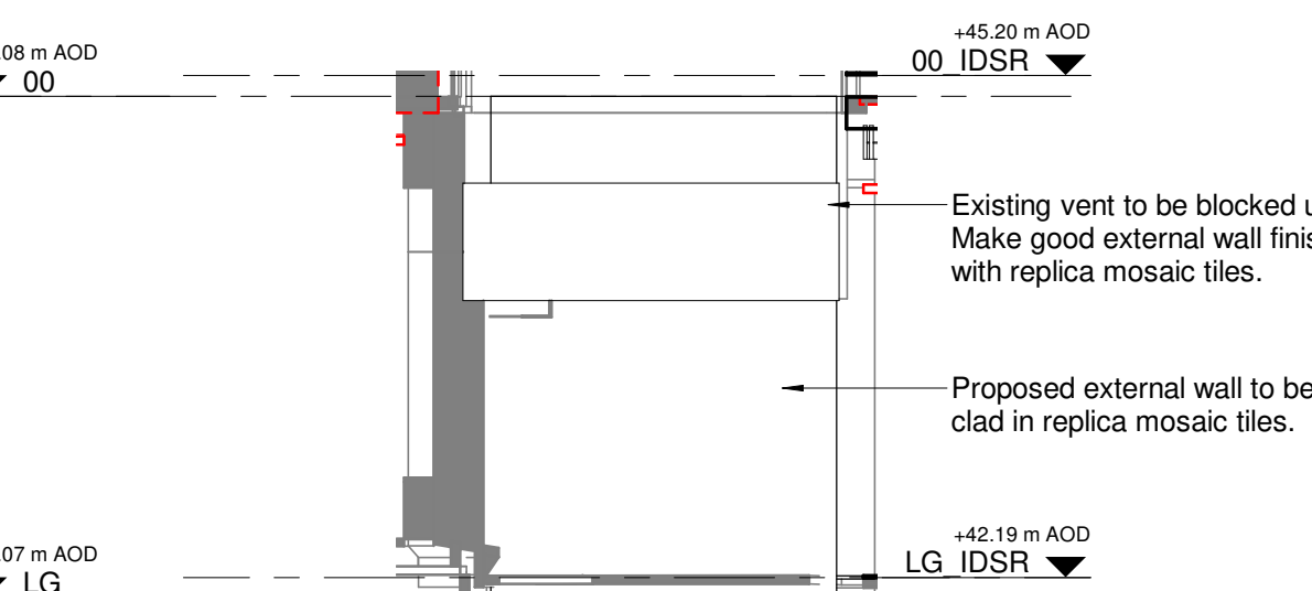
5 External Wall Repair - Proposed Vent Removal 1 : 50
