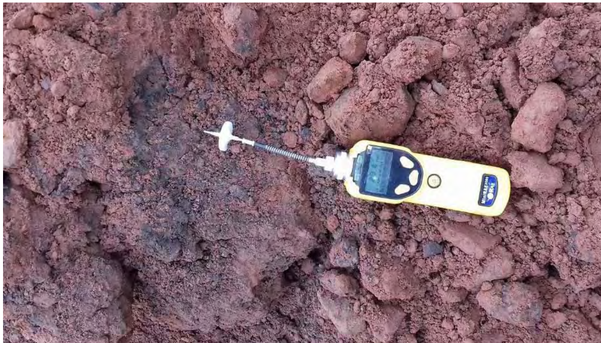
PLATE 4 – PID MONITORING OF CONTAMINATED MATERIAL
