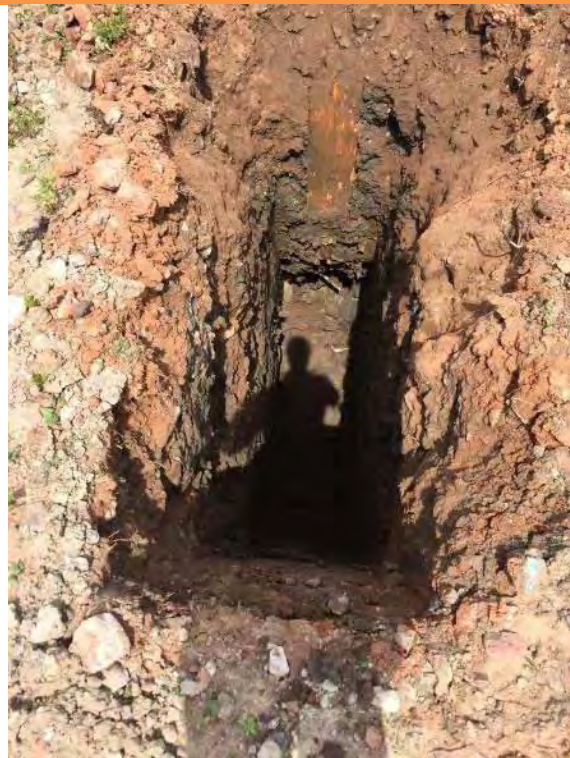
PLATE 16 – SOURCE AREA 2 FURTHER INVESTIGATION TRIAL PIT
