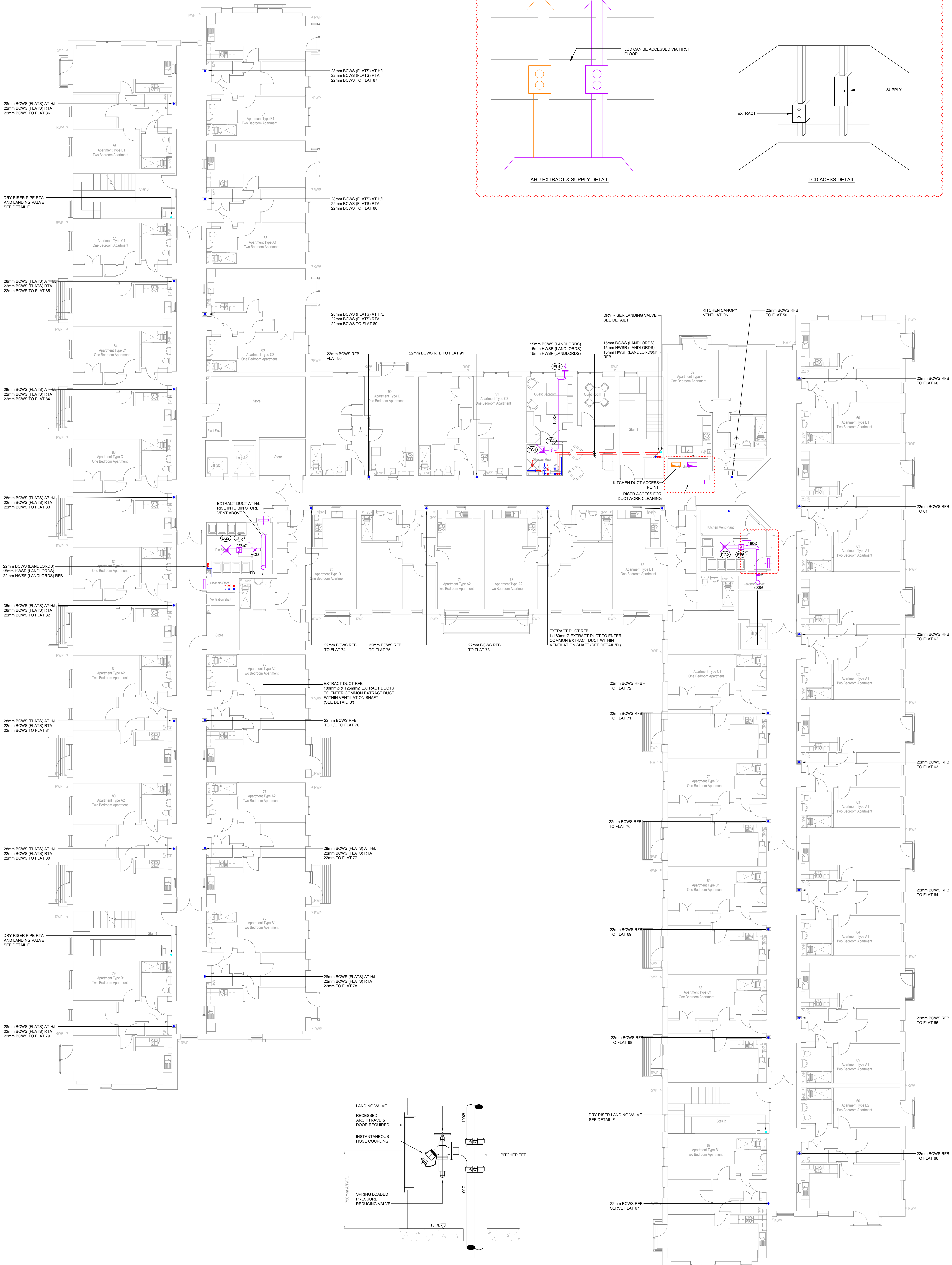
DRY RISER PRESSURE REDUCING LANDING VALVE DETAIL F
