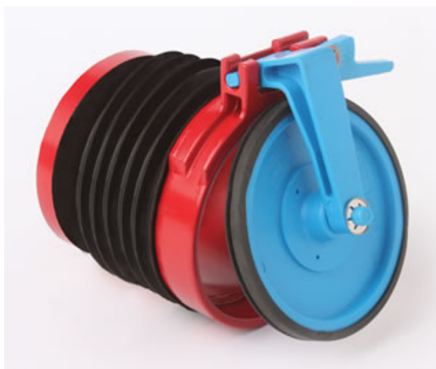
Picture 3: Example of the SMART AirBrick which has been designed to allow air to pass through freely but not water. It features simple flood activated valves that ensure compliance with BS493:1995 as an airbrick but, as soon as water enters the brick, the valves are forced closed preventing flood water from passing through.
