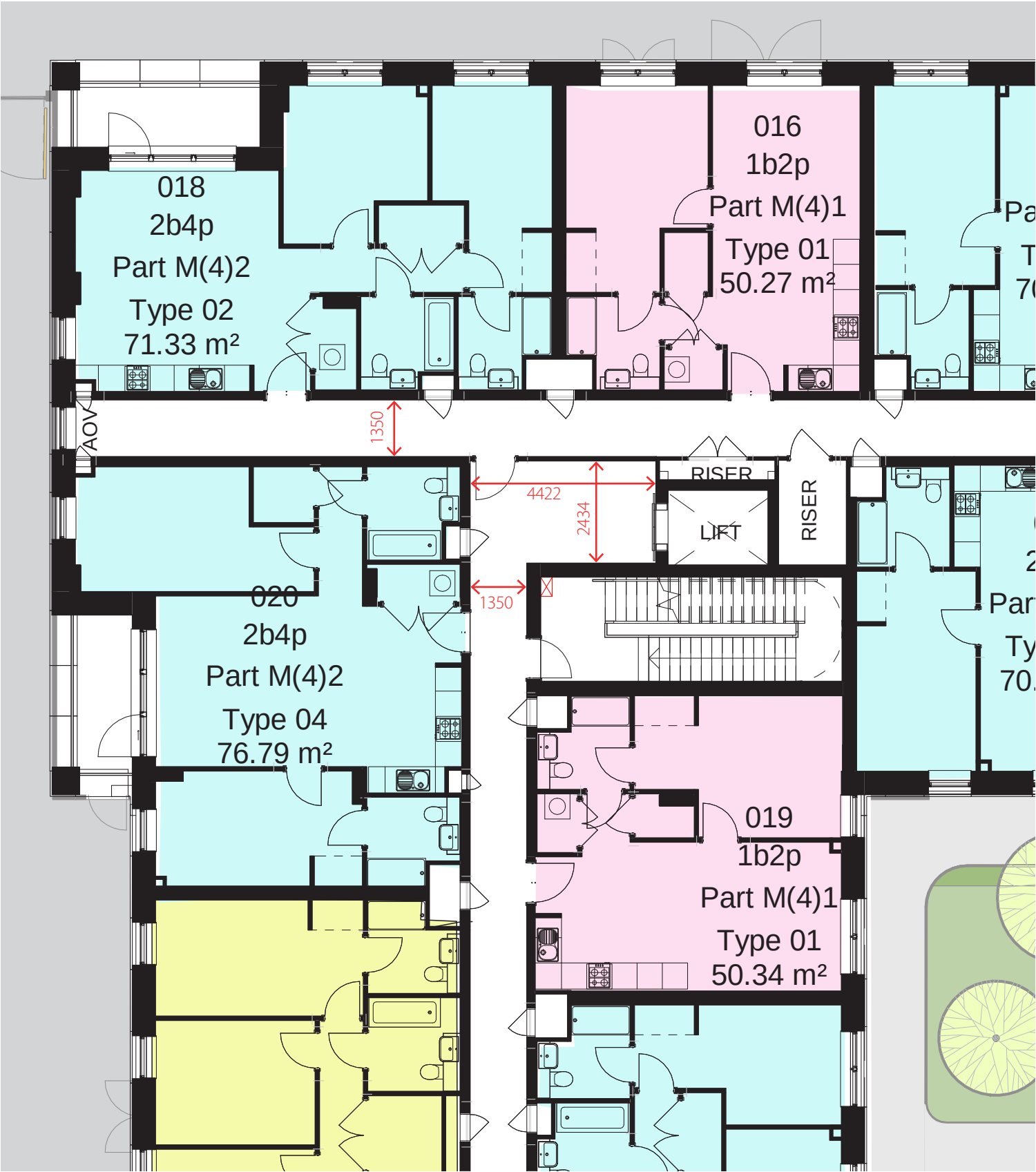
Typical Upper Floor Core Arrangement
