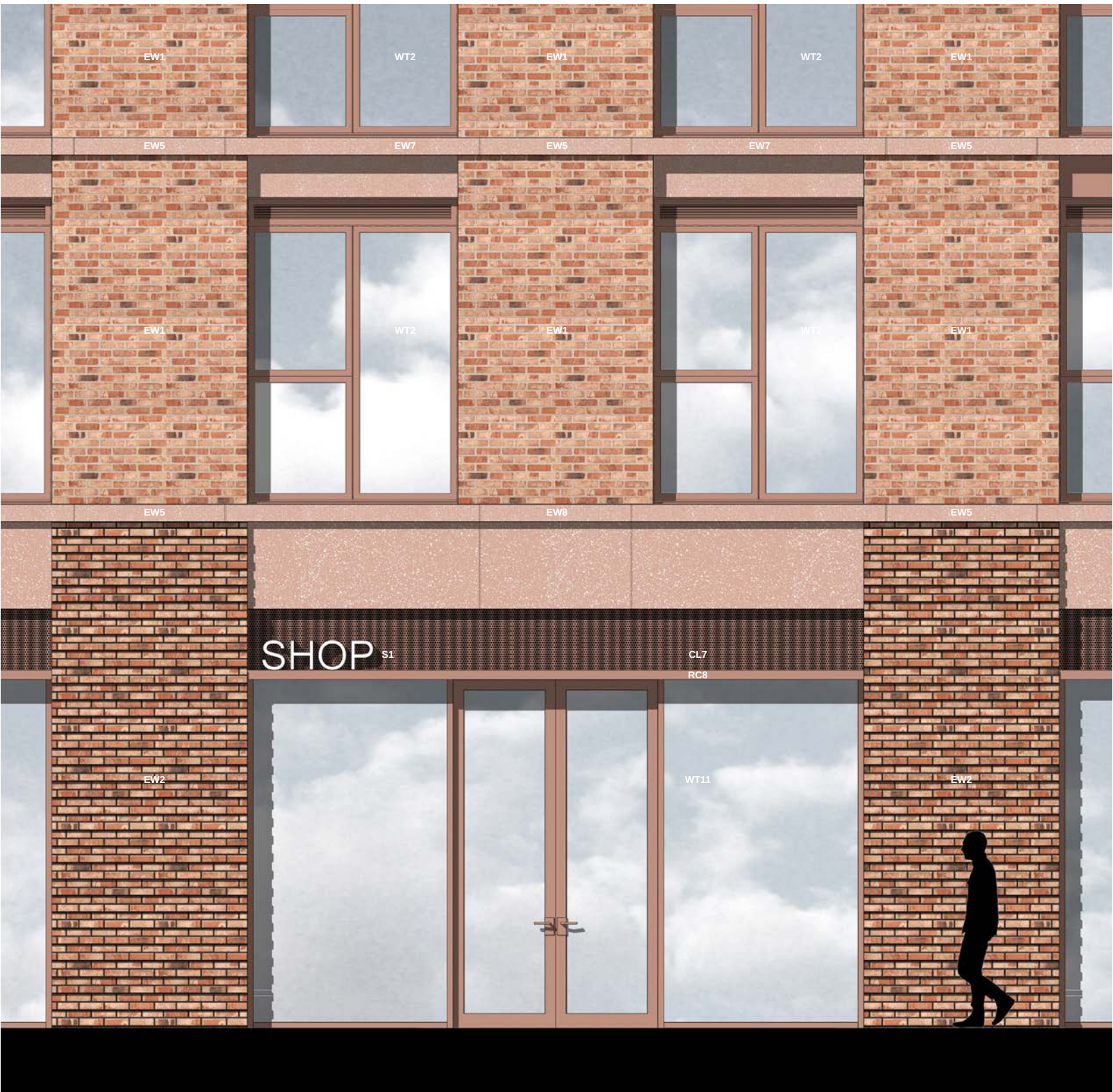
Detailed Section & Illustrative Elevation through Commercial Bay and Typical Residential Window
