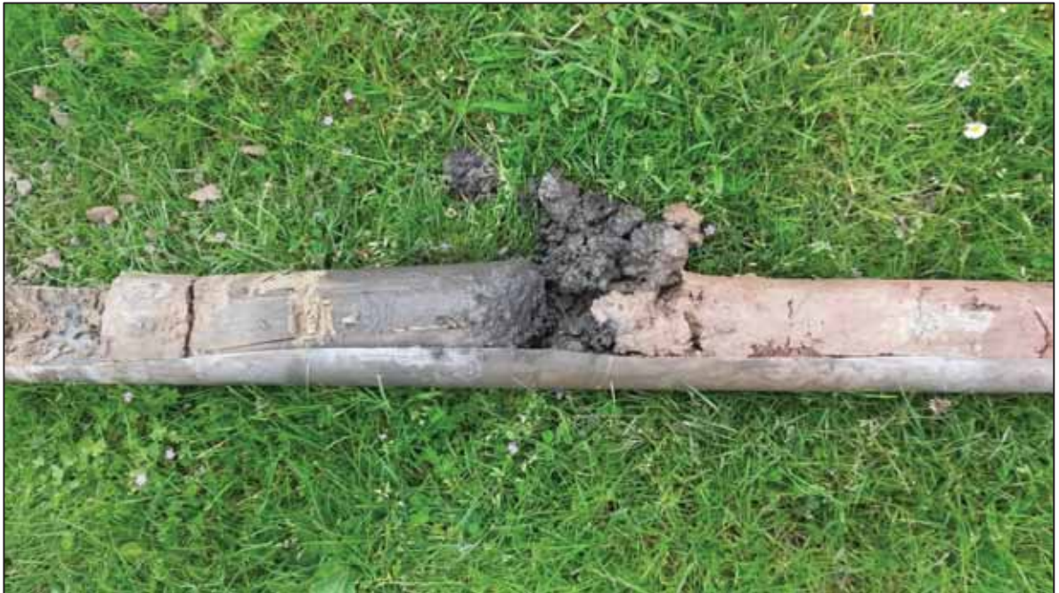
Photograph 1: WS101 showing thin groundwater seepage between Made Ground and bedrock
