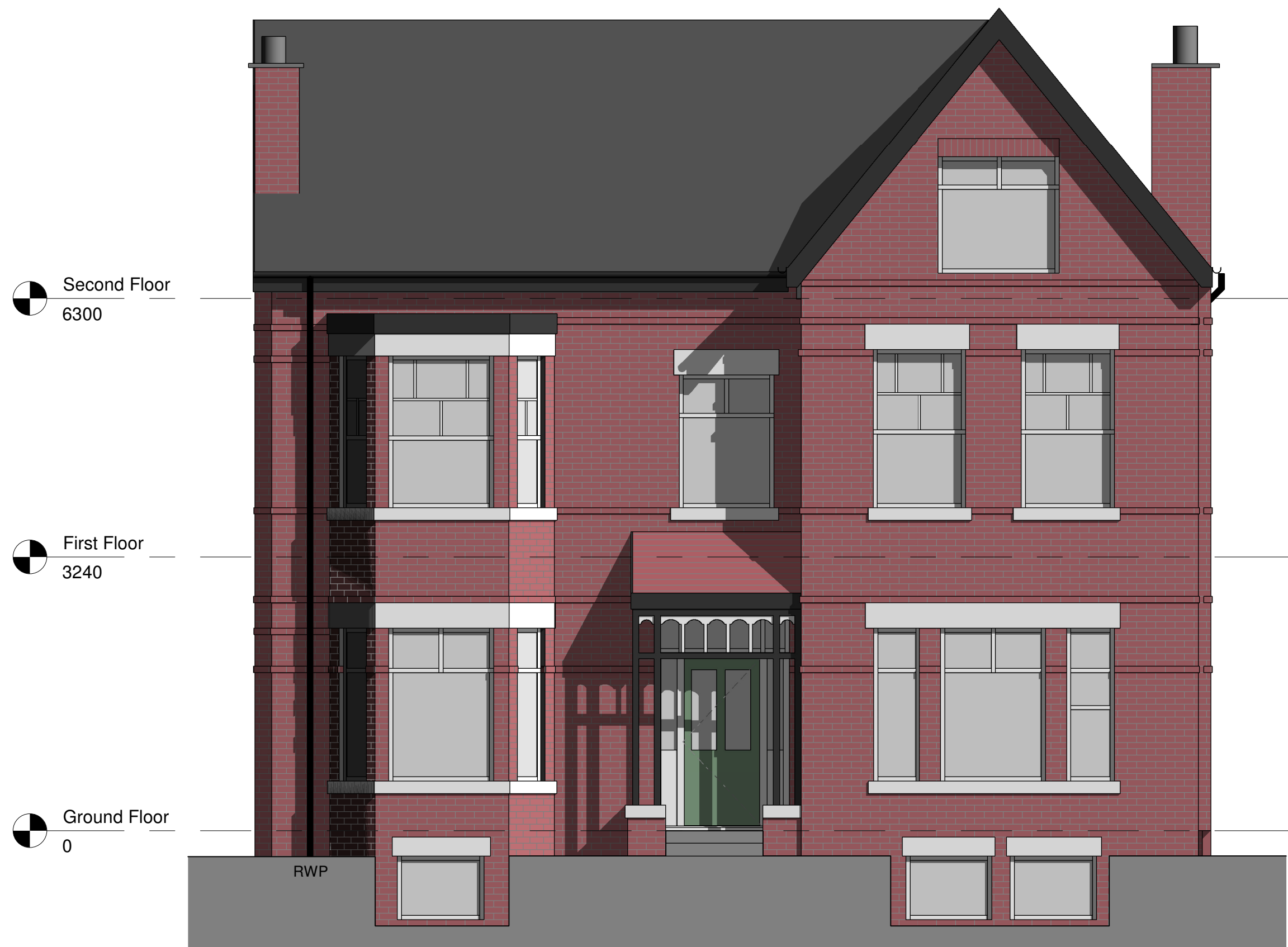
Existing South Elevation 1 : 50
