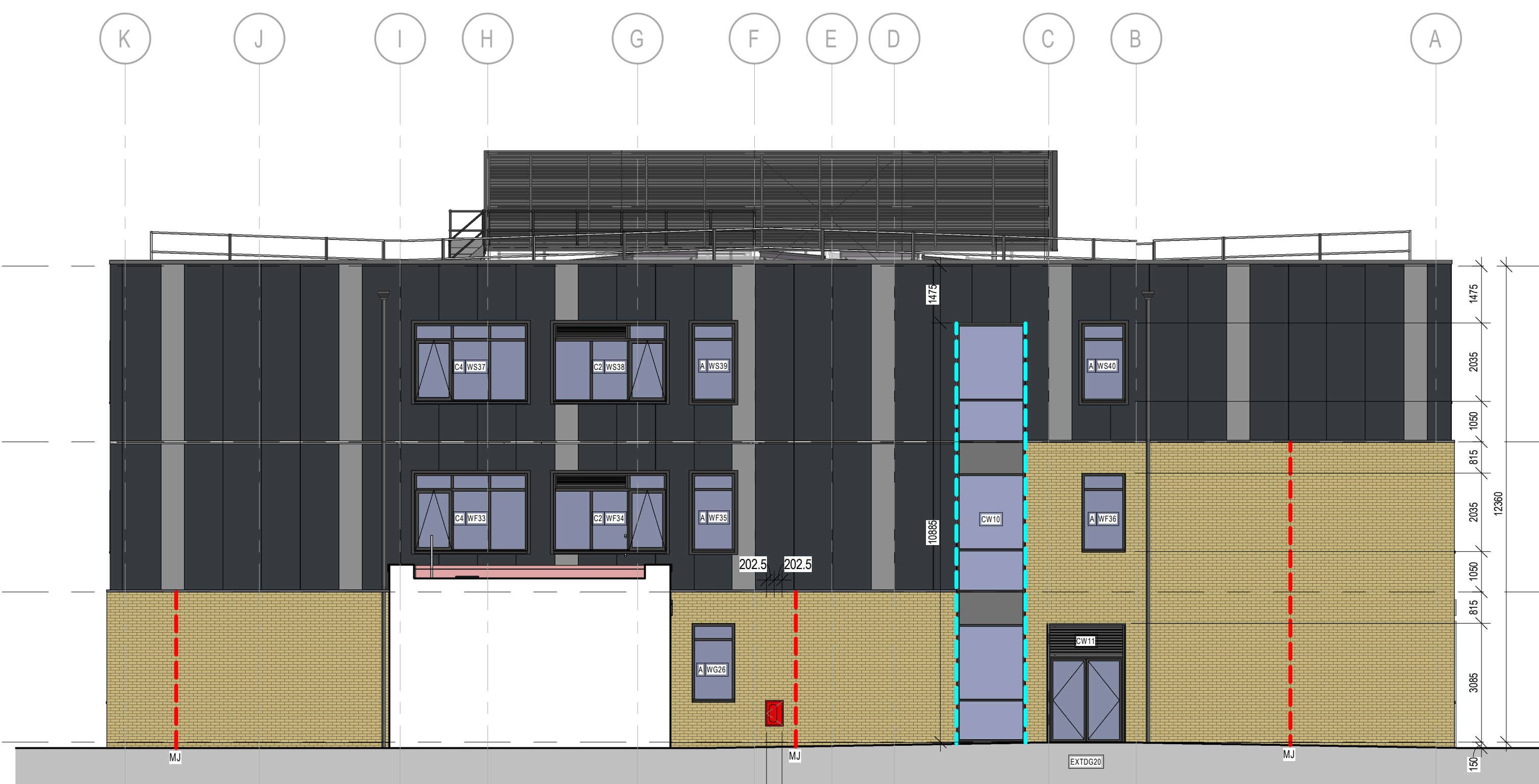
East Elevation GA (Main Building) 1 : 100
