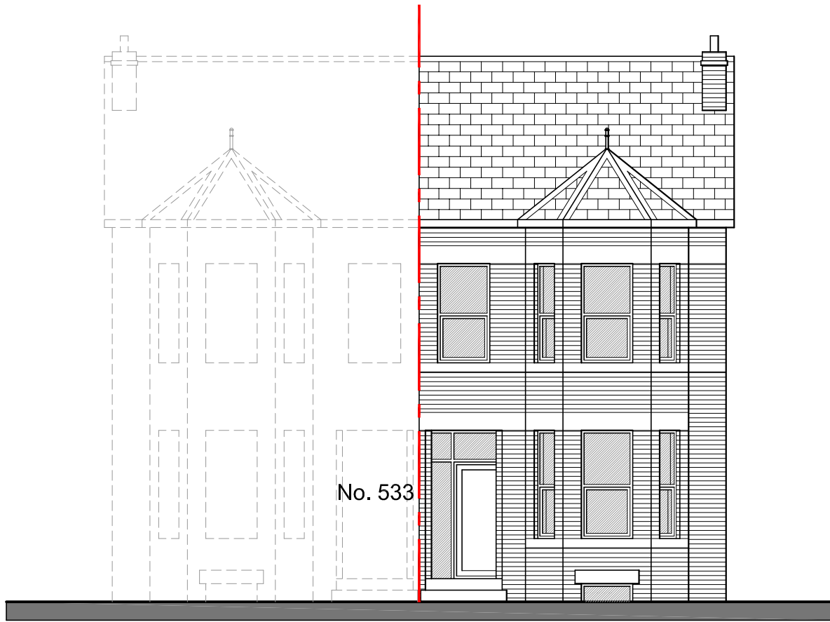
Existing Front Elevation 1:100
