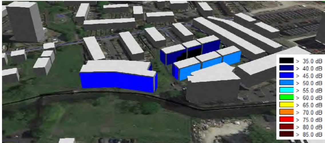
Figure 8 Screenshot of 3D environmental noise model – Predicted facade noise levels, daytime, L_{Aeq} (dB)
