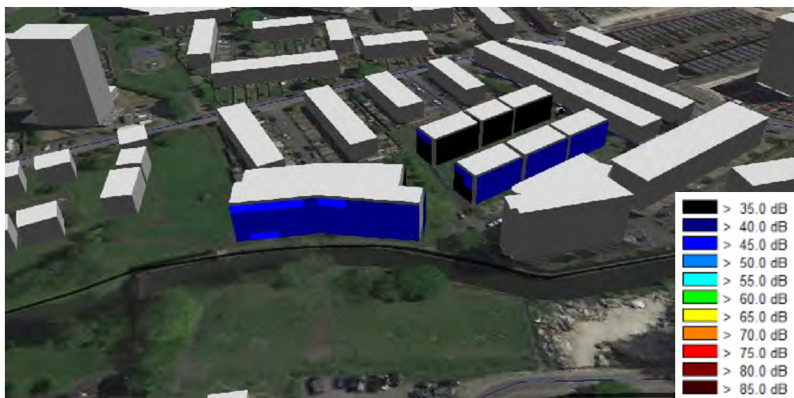
Figure 9 Screenshot of 3D environmental noise model – Predicted facade noise levels, night-time, L_{Aeq} (dB)
