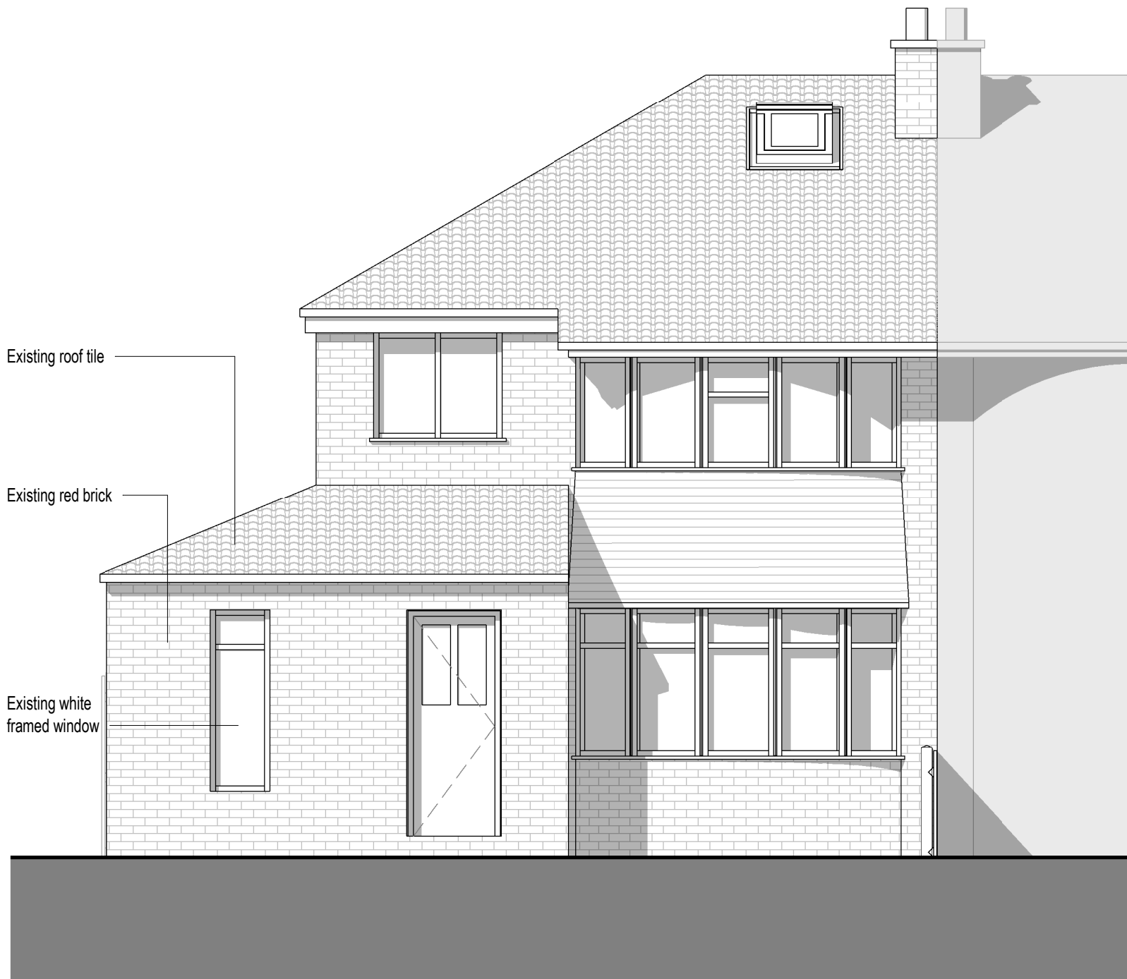
01 EXISTING ELEVATIONS - NORTH-EAST 1 : 50
