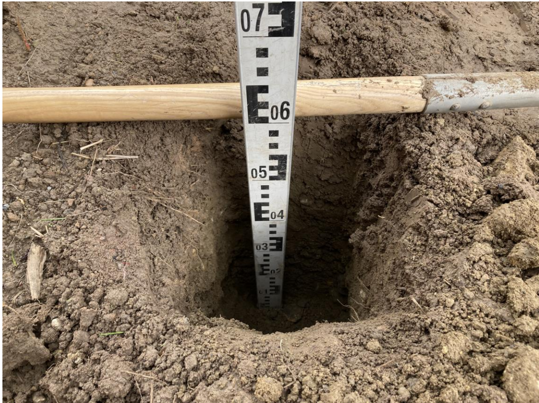
Photograph 1 200mm of topsoil and 400mm of subsoil emplaced in VP01.
