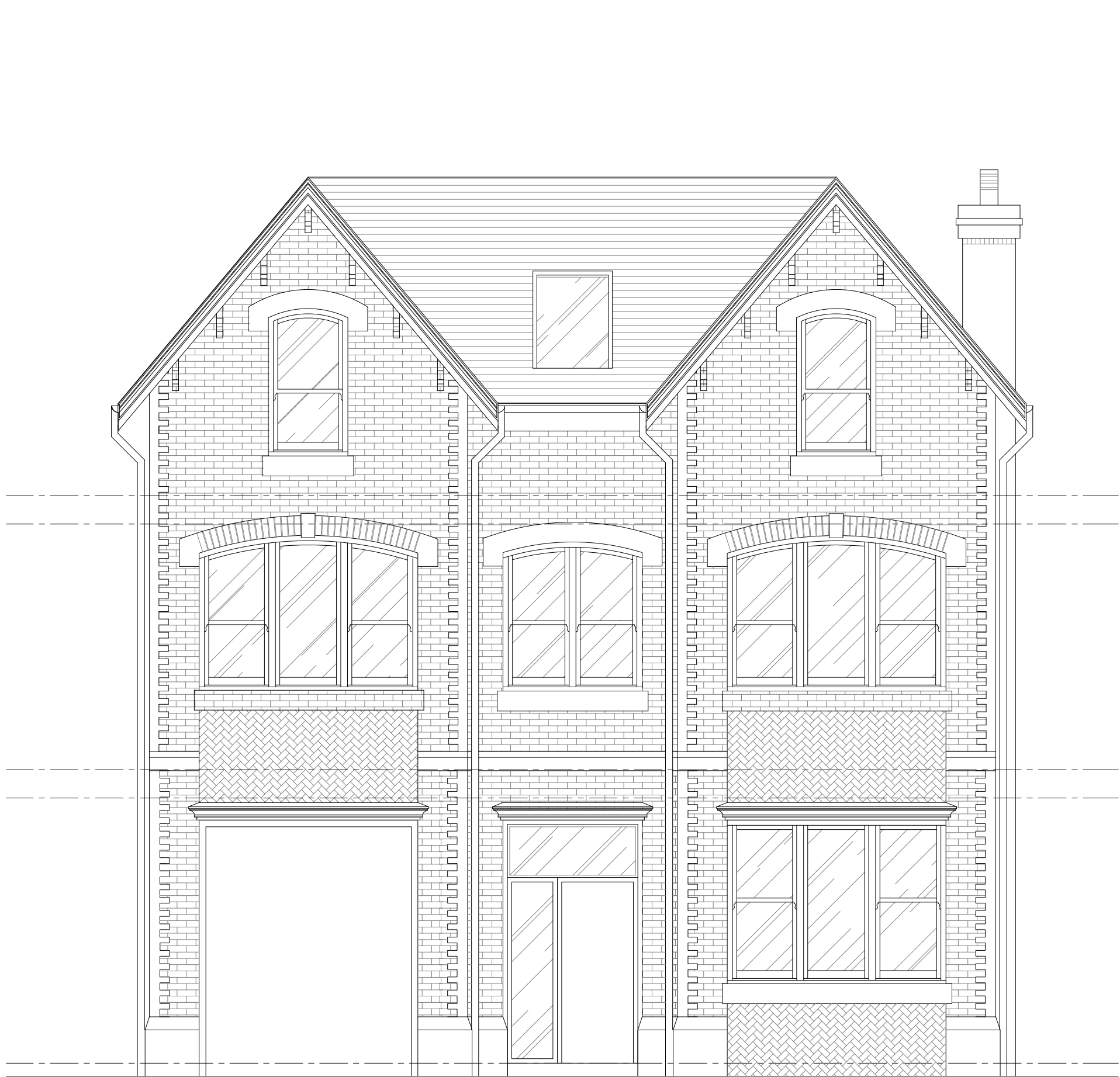
01 160 DETACHED HOUSE FRONT ELEVATION SCALE - 1:50@A1 ELEVATION
