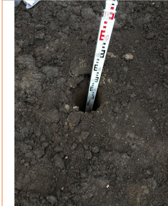
Depth of Cover System at Ground Level
