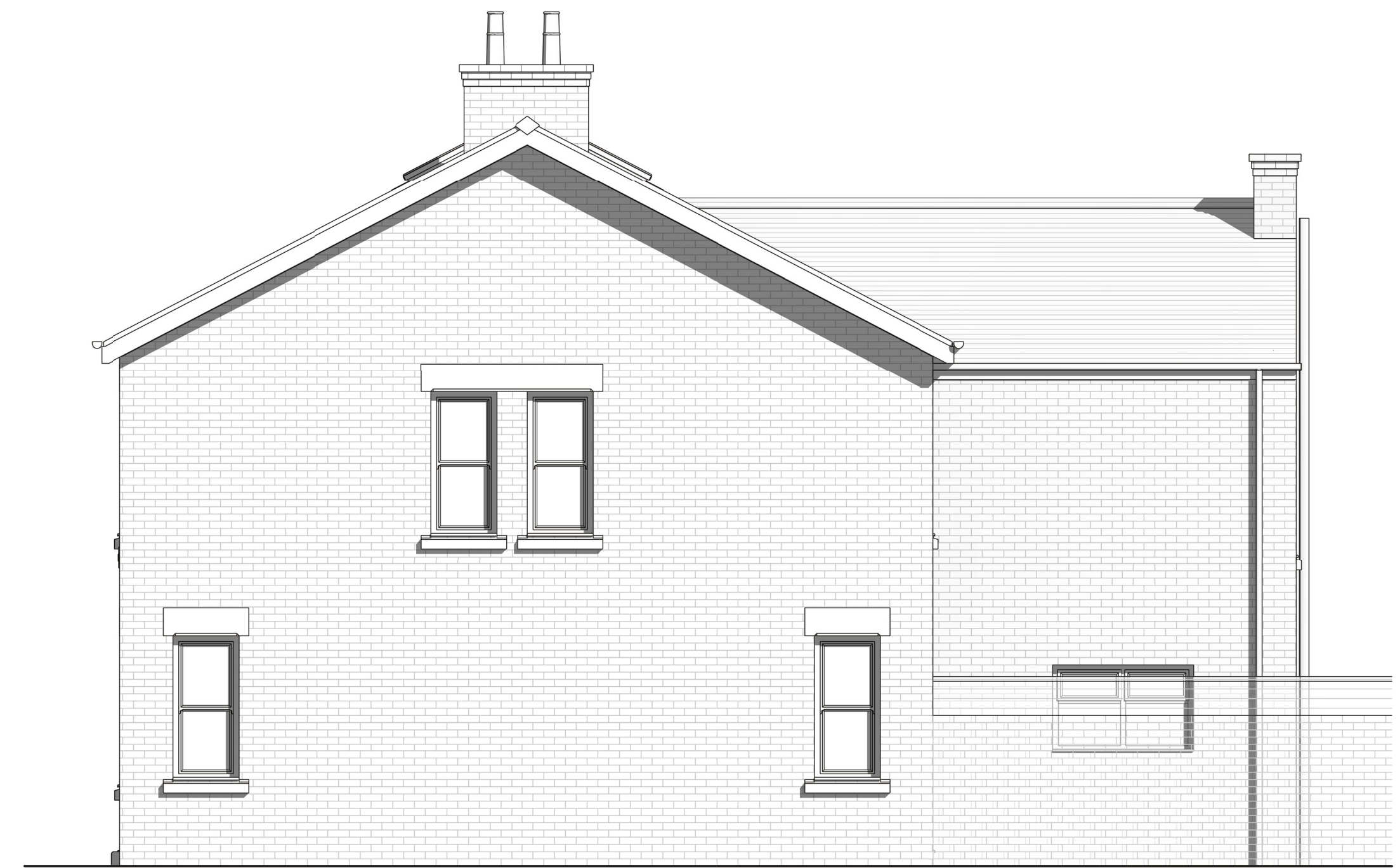
Existing Side Elevation 1 : 50
