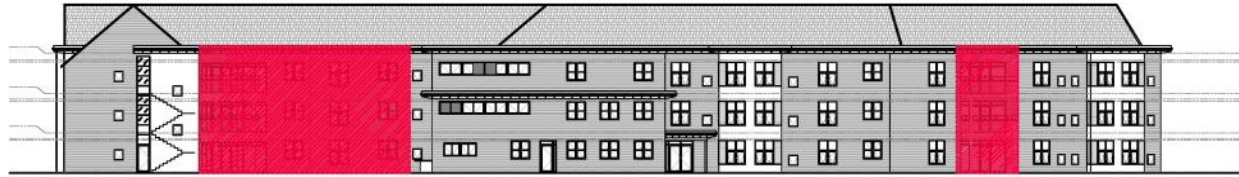
WEST ELEVATION- DEMOLITION AREA
