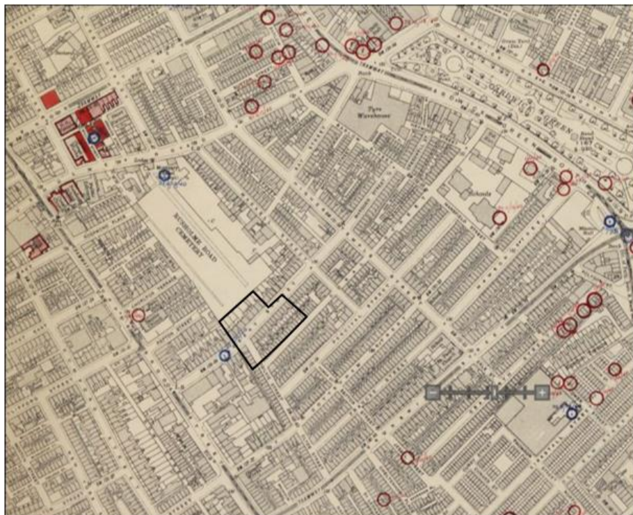
Figure 2.6 – WWII Bomb Damage Mapping (site boundary shown in pink). Red circles for fire bombs; blue circles for high explosives; pink shading for damaged buildings; red shading for demolished buildings; green marks: line mines, indicating bomb damage by the Luftwaffe during the Blitz
