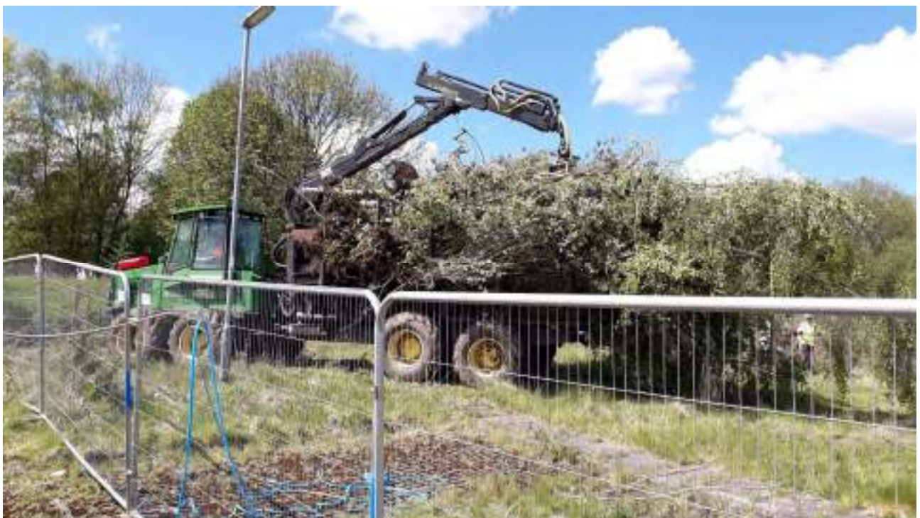
Figure 6 : A forestry forwarder being used to collect and stockpile felled timber
