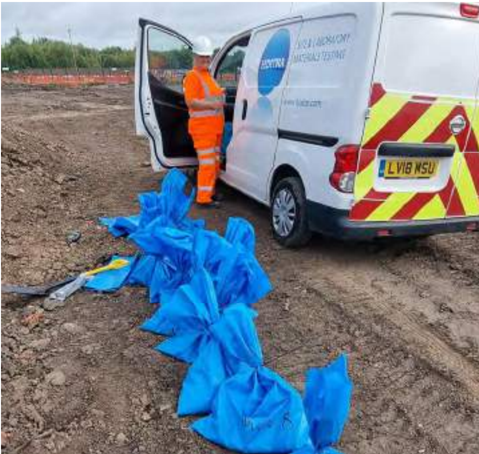
Figure 50 : Collection of bulk soils samples for laboratory analysis
