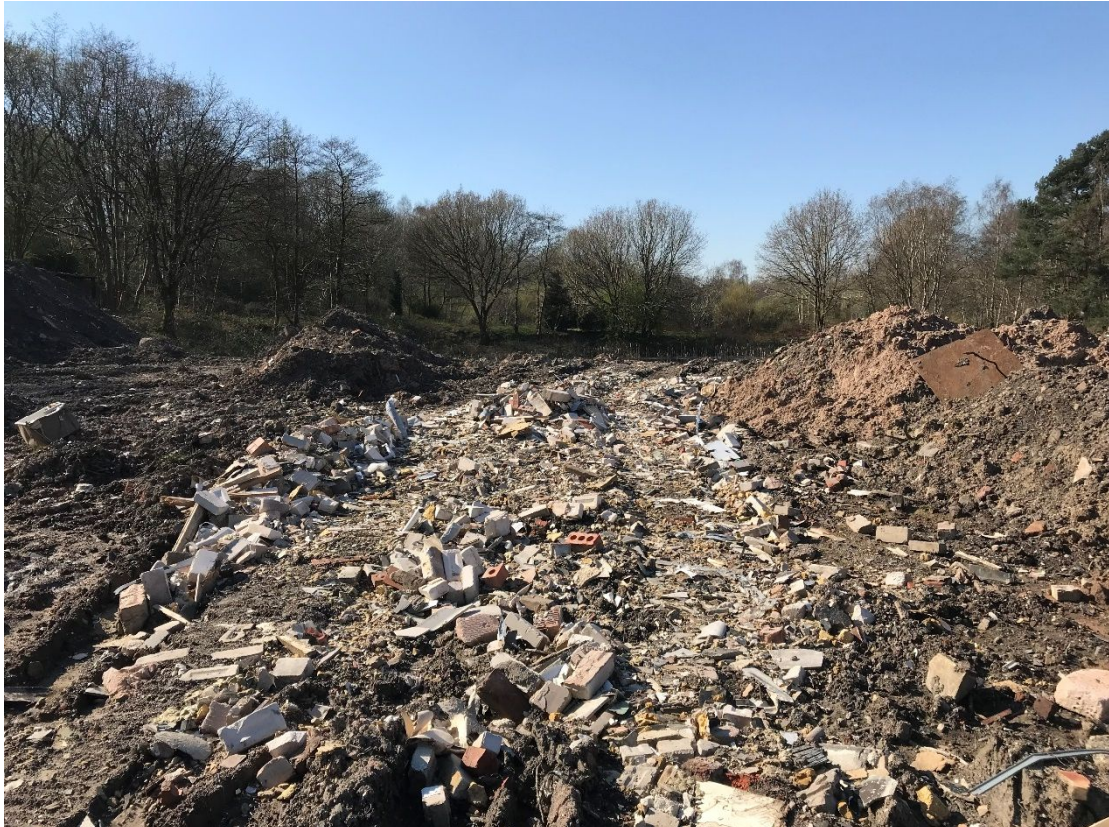
Plate 6-1: Visible pieces of likely ACMs on the site surface.
