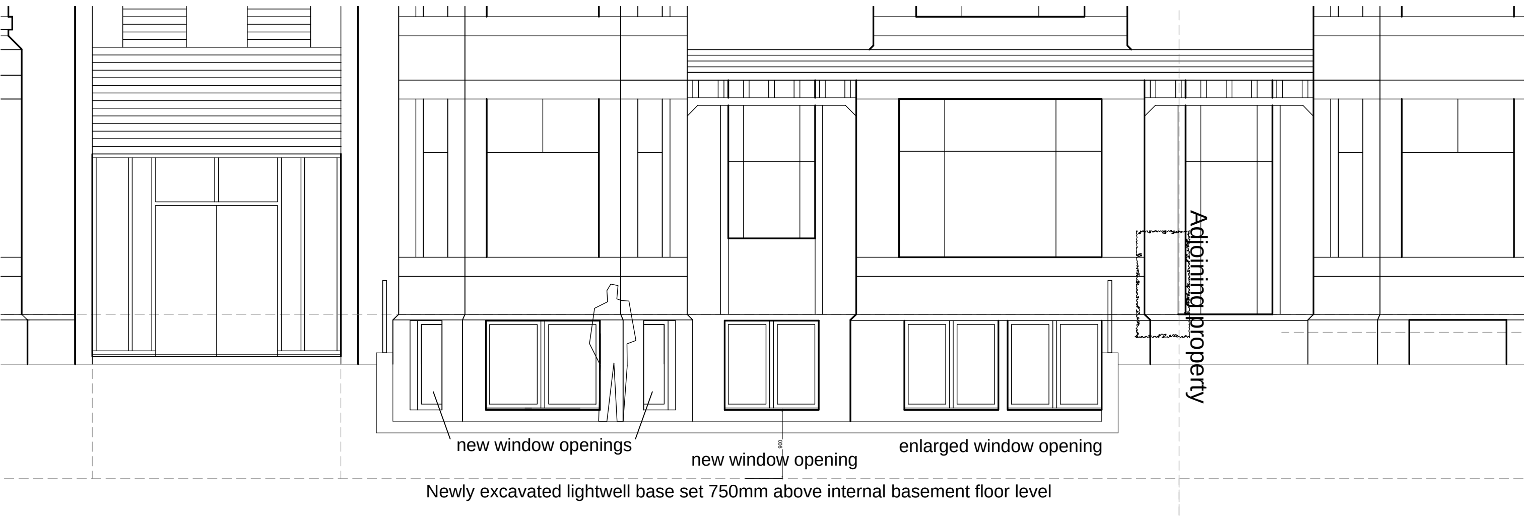
Front elevation to Wilmslow Road within lightwell
